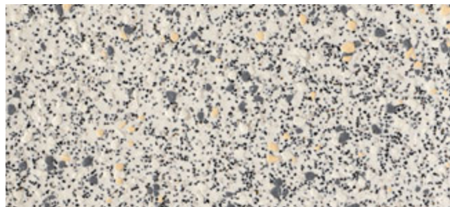
Flooring shows no visible marking after gel left for 24 hours and removed only with water.
